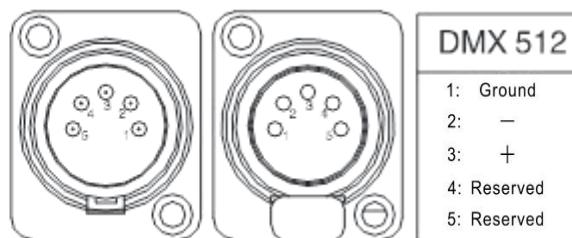
Connect the Console's DMX OUTPUT to the first fixture's DMX INPUT, then the first fixture's DMX OUTPUT to the second fixture's DMX INPUT and so on. It is recommended not to connect more than 32 units on a single
