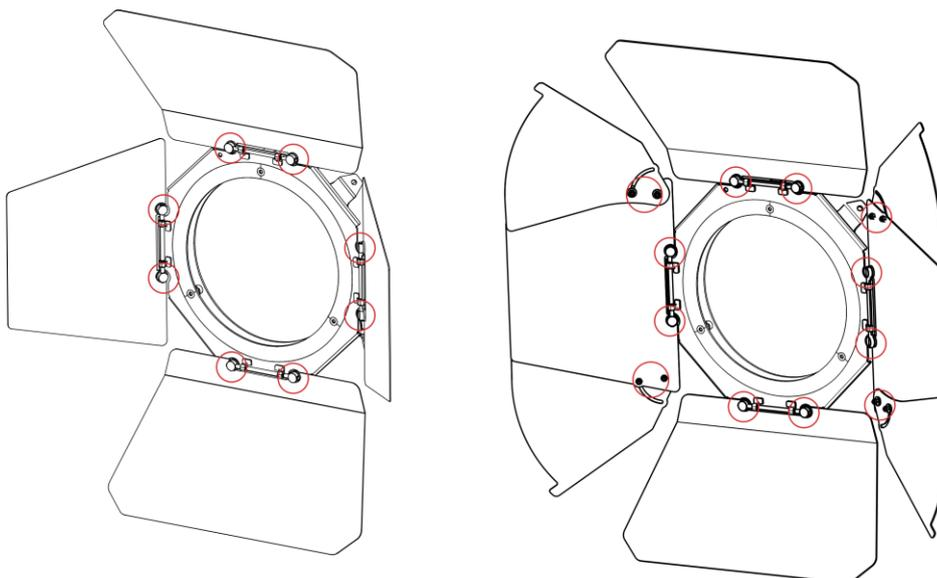
It is possible to adjust the resistance of the blades by loosening or tightening the nuts
