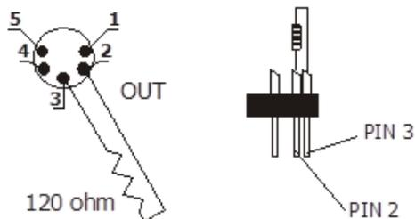
Place a 120  $\Omega$  resistor between pin 2 and 3 of a male XLR connector;
