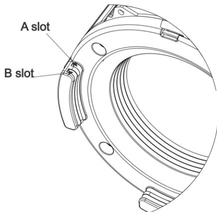
**SAFETY CABLE SLOT FOR INSTALLATION WHERE NECESSARY**
