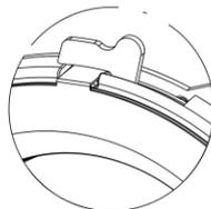
The gel holder must only be inserted in position A
